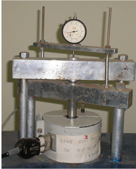
Fig. 2 Photographic View of Cyclic Swell Shrink Test Set-Up
