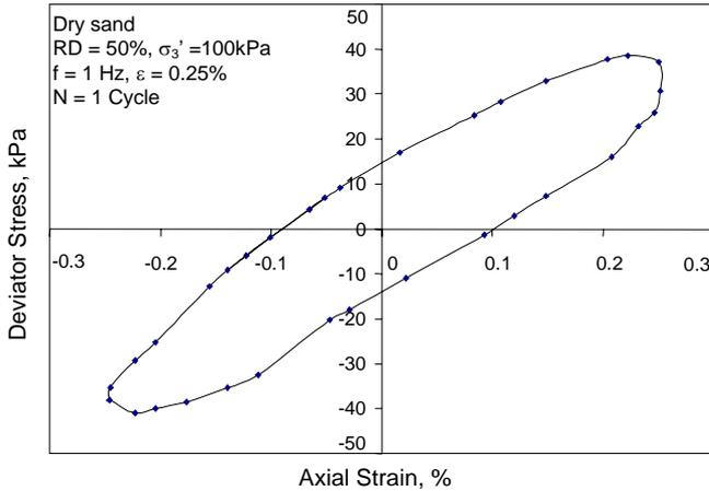
**Fig. 5 Deviator Stress Versus Axial Strain Relationship at First Cycle for Sand Sample at Relative Density of 50%**
