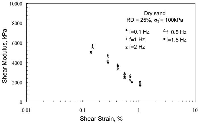
**Fig. 10 Influence of Frequency on Shear Modulus for Dry Sands**
