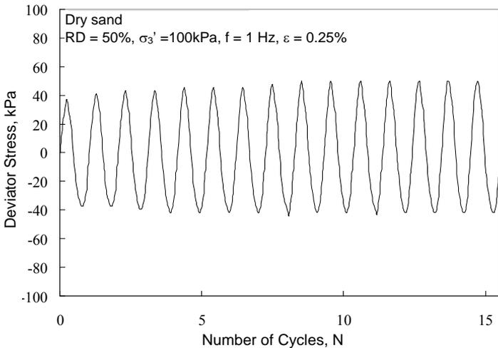
**Fig. 4 Deviator Stress Versus Number of Cycles for dry Sand at Relative Density of 50%**
