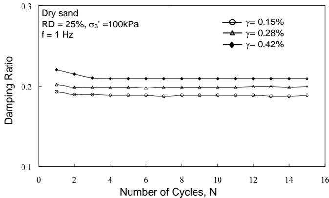
**Fig. 7 Relationship Between Damping Ratio and Number of Cycles at 25% Relative Density for Dry Sand**
