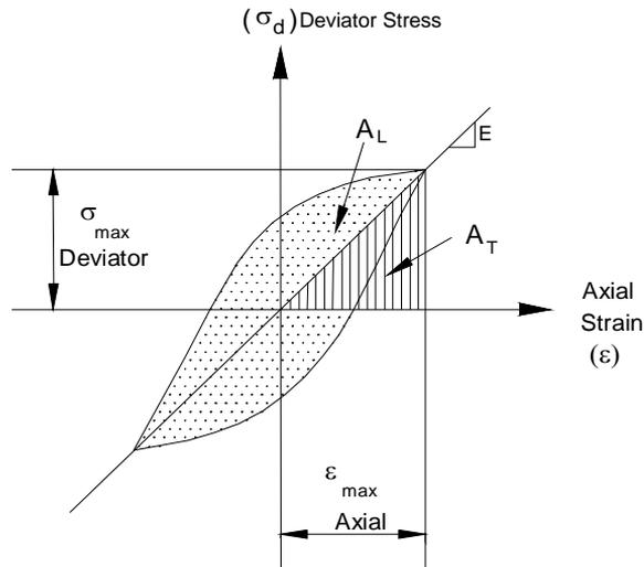
Fig. 2 Hysteretic Stress-Strain Relationship for Cyclic Loading
