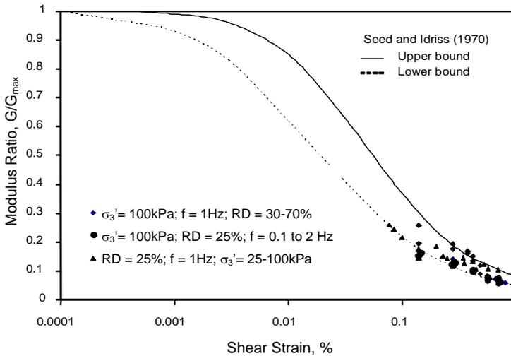
**Fig 12. Variation of Modulus Ratio with Shear Strain for Different Parameters Considered for the Present Investigation**
