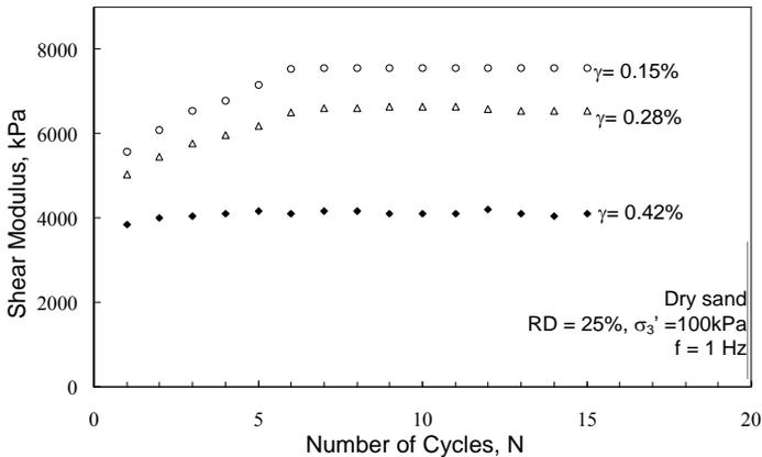
**Fig. 6 Relationship Between Shear Modulus and Number of Cycles at 25% Relative Density for Dry Sand**
