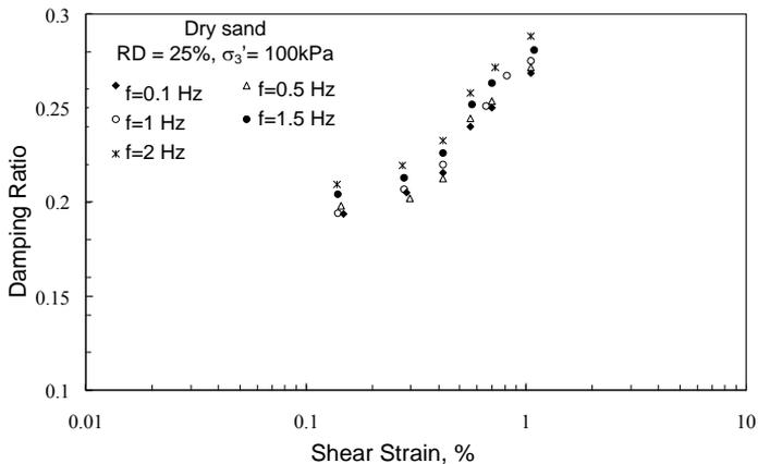
**Fig. 11 Influence of Frequency on Damping Ratio for Dry Sand**
