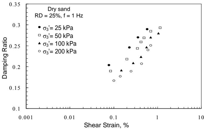
Fig. 9 Influence of Confining Pressure on Damping Ratio for Dry Sands
