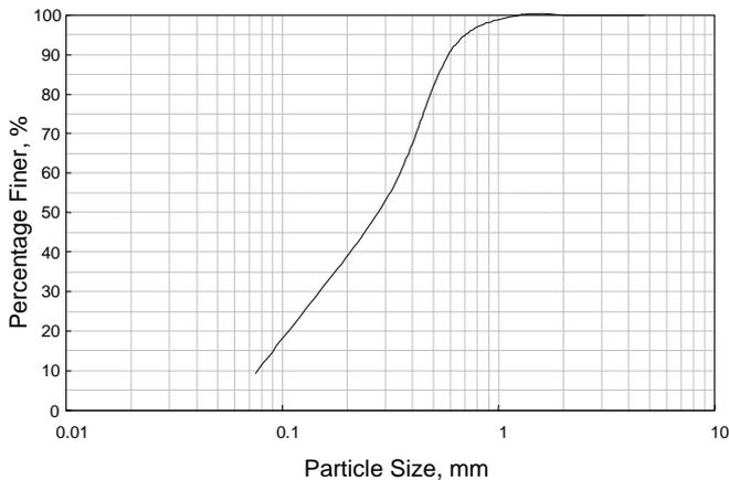
**Fig. 1 Particle size distribution curve**
