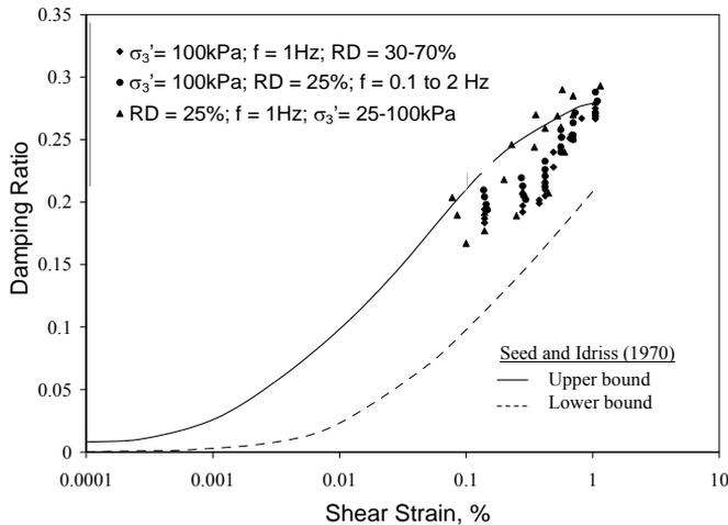
**Fig 13. Variation of Damping Ratio with Shear Strain for Different Parameters Considered for the Present Investigation**
