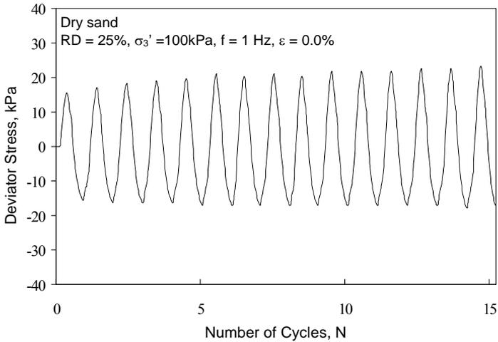
**Fig. 3 Deviator Stress Versus Number of Cycles for Dry Sand at Relative Density of 25%**
