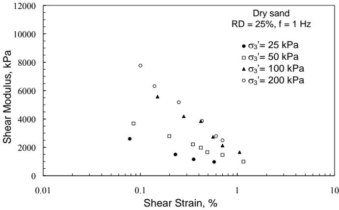
Fig. 8 Influence of Confining Pressure on Shear Modulus for Dry Sands
