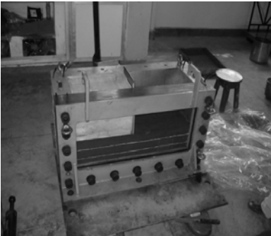
a) Soil model constructed with a guiding box to align the sheet pile wall
