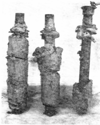
Fig. 18 Photograph of pulled out Anchors – Type I, Set I, Soil I
