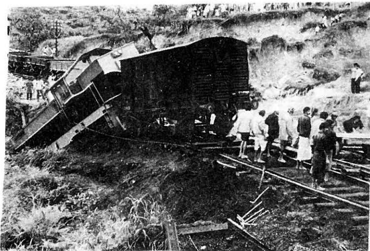
FIGURE 69 Derailment of Goods Train at Watawala on 3rd June 1992 due to Earth-Slide
