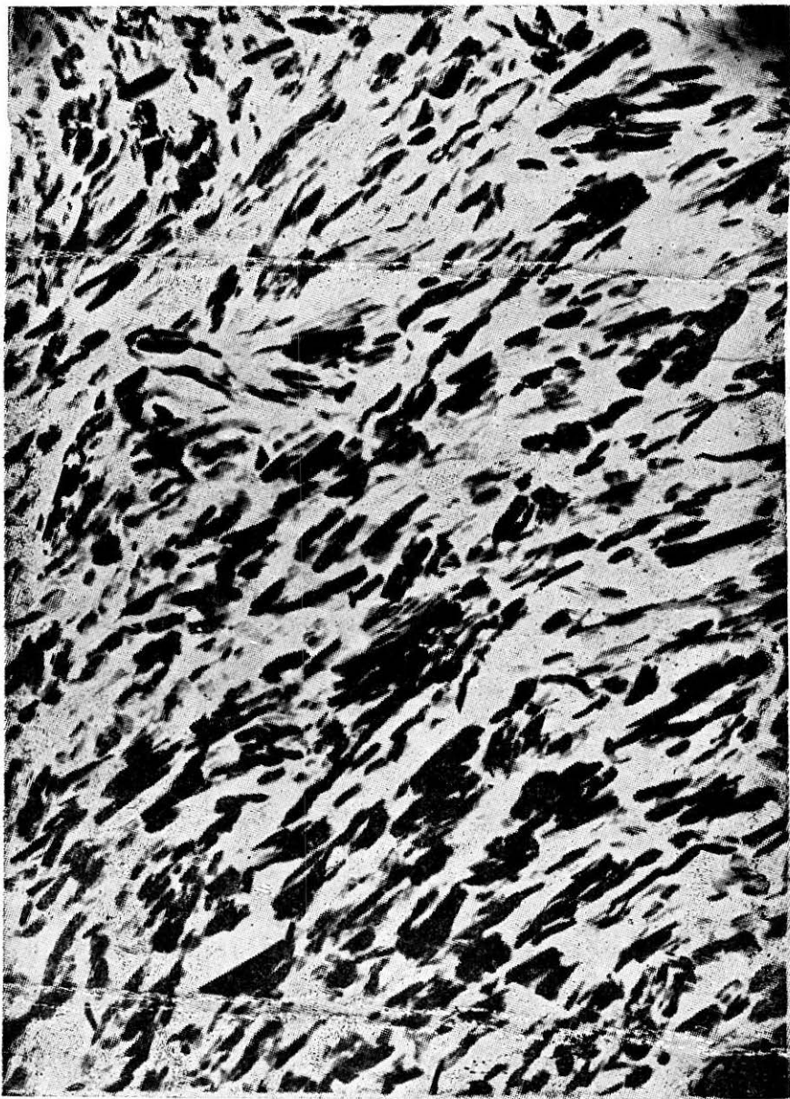
FIGURE 2 : Araldite AZ 15 impregnation of Kaolin. Max Consolidation load 45 kg/cm 2 . Thickness of the ultra-thin section 900 A°. Diamond Knife.
